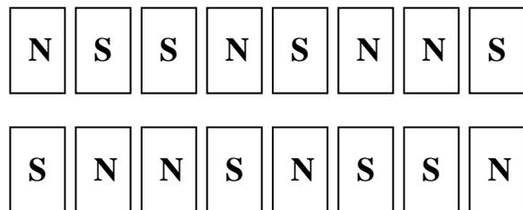
arrangement can be read later by scanning the disk with the same arm. Each bunch of molecules is called a BIT. Groups of them are called BYTES. This drawing is an 8-bit byte. As the molecules flip over, they represent a 1 or a 0. The north magnetic pole is 1, the south is 0. Digital storage always involves just 2 values; 1's and 0's, or on and off. Our drawing is the number 10010110. If we use a special number system called binary numbers, these 8 bits store the number as 140.
